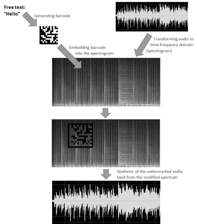
Figure 2. Watermarking process using the Spectral Barcode Audio Watermarking (SBAW) technique
