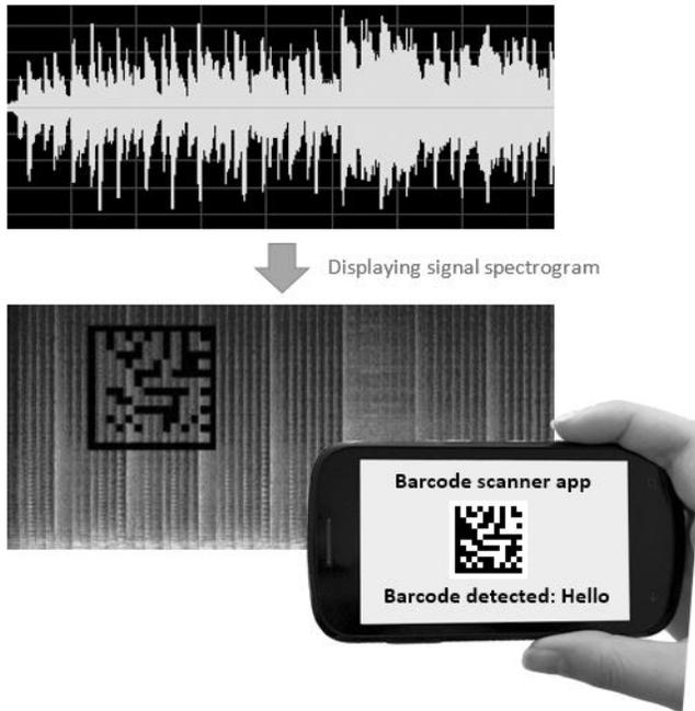
Figure 3. Watermark extraction from signal spectrogram using barcode reader
